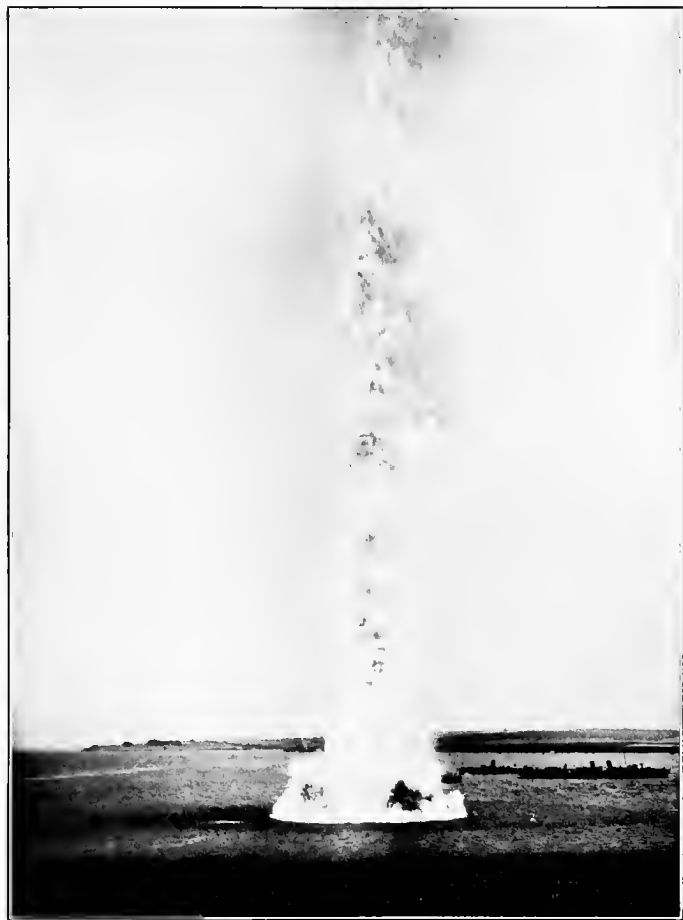
The explosion, eight feet under water, of a naval defense mine containing 161 lbs. of wet gun cotton
